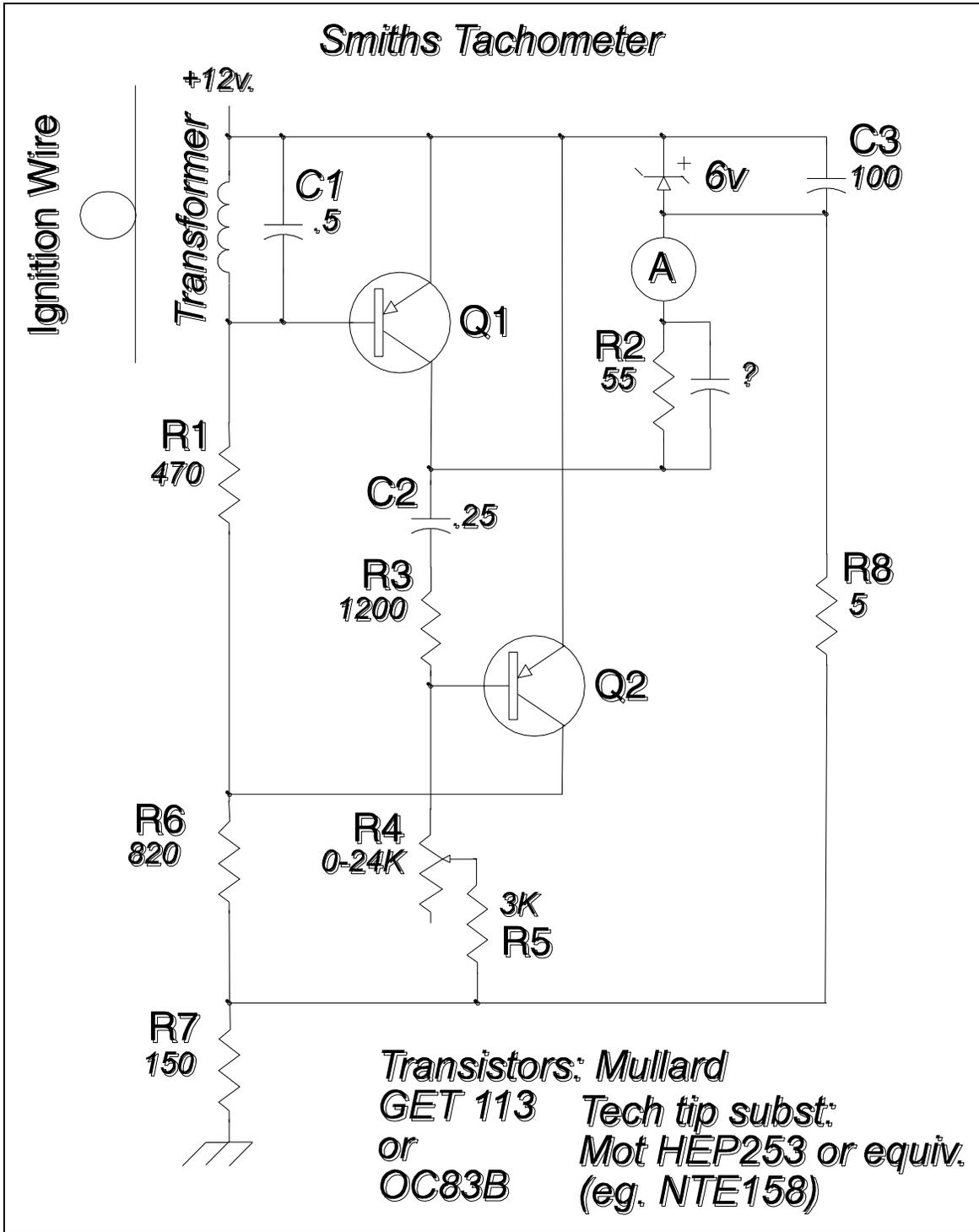
The two transistors together form a monostable multivibrator, or one-shot. Normally, the collector of Q1 is at 6V. An ignition pulse couples through the transformer to trigger a
