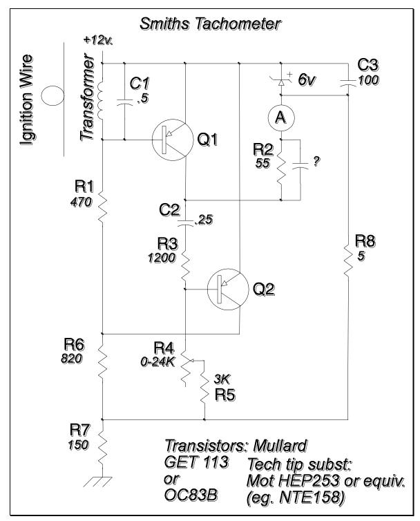
The two transistors together form a monostable multivibrator, or one-shot. Normally, the collector of Q1 is at 6V. An ignition pulse couples throough the transformer to trigger a
