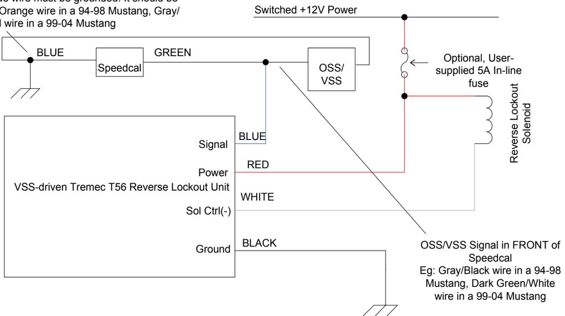
**VSS/OSS Connection Diagram (for general electronic speedometer cars):**
