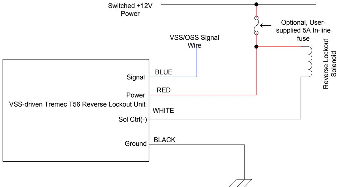
Hall Effect sensors such as those used in Dodge Vipers generate a 0-5 or 0-12V square wave signal which is not directly compatible with our Lockout Units. To use the Accutach Co. T56 OSS/VSS Reverse Lockout Unit with a Hall Effect speed sensor, simply put a 22uF, 25V capacitor in series between the Hall Effect signal and the BLUE input wire to the Lockout Unit.
