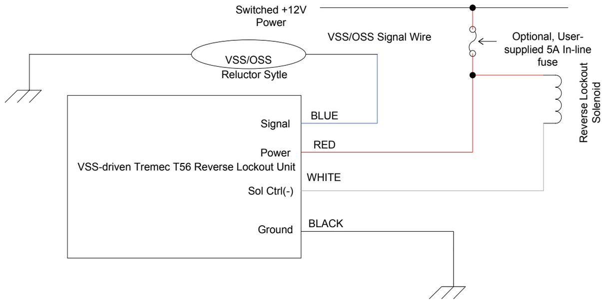
Hall Effect sensors such as those found in Dodge Vipers generate a 0-5 or 0-12V square wave signal which is not directly compatible with our Lockout Units. To use the Accutach Co. T56 OSS/VSS Reverse Lockout Unit with a Hall Effect speed sensor, simply put a 22uF, 25V capacitor in series between the Hall Effect signal and the BLUE input wire to the Lockout Unit.
