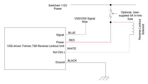
Hall Effect sensors such as those used in Dodge Vipers generate a 0-5 or 0-12V square wave signal which is not directly compatible with our Lockout Units. To use the Accutach Co. T56 OSS/VSS Reverse Lockout Unit with a Hall Effect speed sensor, simply put a 22uF, 25V capacitor in series between the Hall Effect signal and the BLUE input wire to the Lockout Unit.
