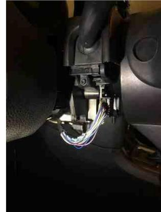
Locate the WH Cruise Button Signal wire and cut it, leaving enough room to slice the Cruise Button Box input wire to the clockspring side of the wire.
