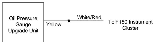
If you did not replace the F150 OEM oil pressure switch with the Autometer sensor, you can simply leave the yellow wire from the upgrade unit unhooked and the OEM switch will drive the idiot light.
