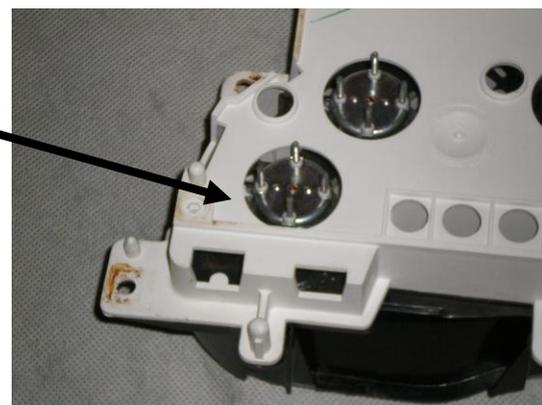
Your new Accutach Co. Oil Pressure Gauge Upgrade Box has 4 wires that must be connected to the pins of the oil pressure gauge. Those pins must be isolated from the electronics on the cluster PCB. If both the PCB electronics and the Upgrade Box are connected to the gauge together, then the upgrade will not work, and the cluster and Upgrade Box may be damaged or destroyed.
