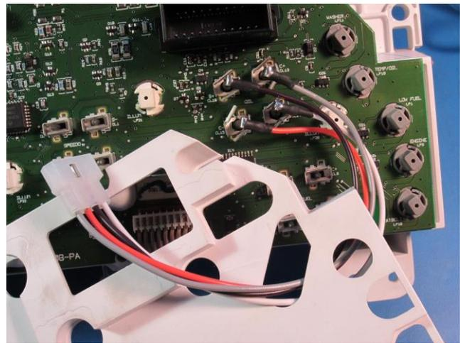
The F150 instrument cluster Hot in Start & Run power is the RD/LG wire and the Hot in Run power is the GY/YE wire.
