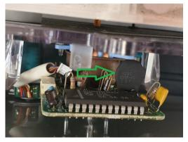
Unfortunately, when these MOVs fail due to old age, they usually short out straight to ground. The fuse for the Always-Hot circuit is too large to protect the instrument cluster. As a result, the Always-Hot PCB trace on the back of the instrument cluster often burns out but sometimes the fuse will blow. Here is a photo of a typical burned trace (circled in green):
