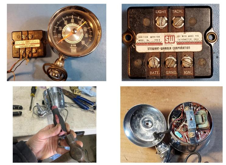
To disassemble the tachometer, carefully tap the bezel off the front of the tachometer at the 4 dimples in the bezel until it is free. Then remove the screw that holds the back on. Removing the two nuts on the back will free the tachometer works from the case to get at the electronics and the ammeter.
