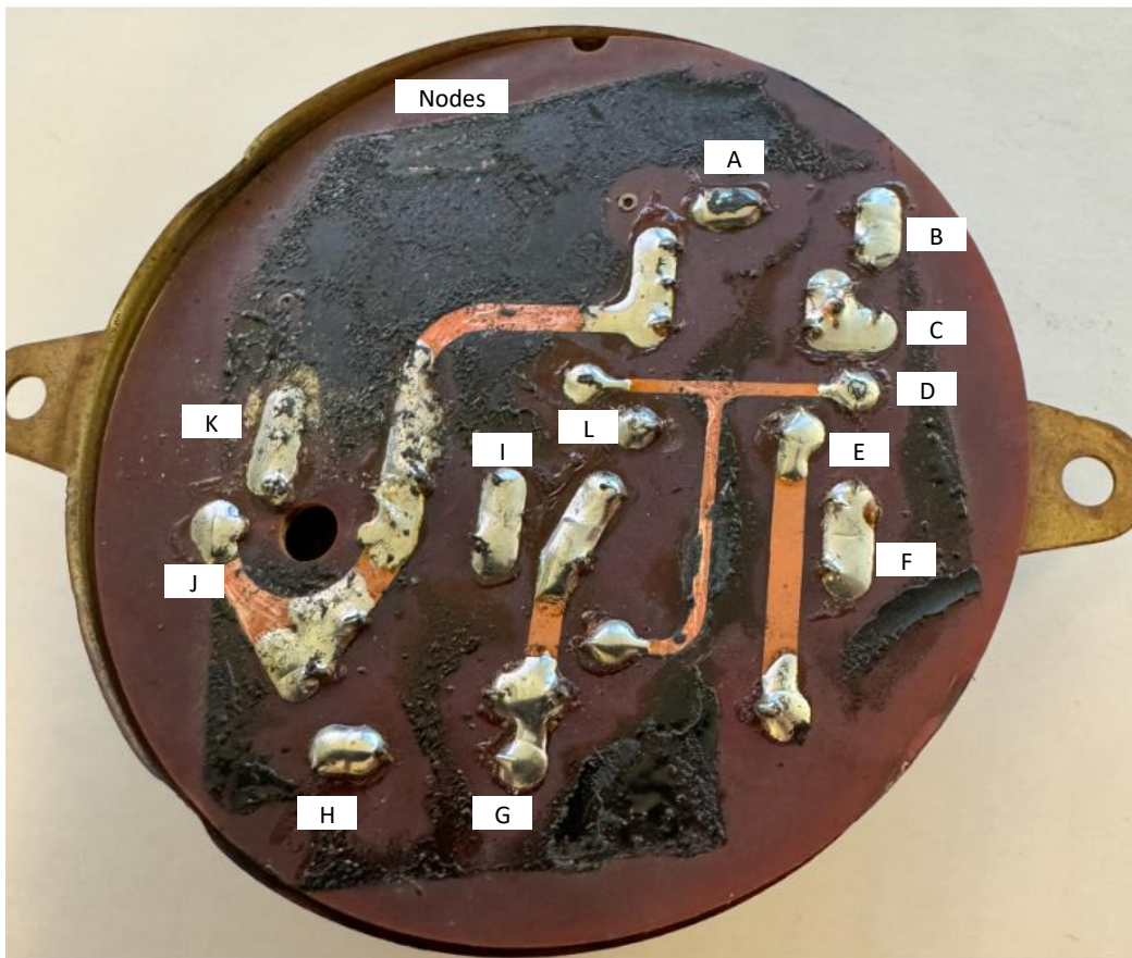
PCB Bottom View is Mirror Image
