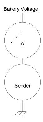
Changing battery voltage is compensated for by the sender. As the voltage goes up, the current also goes up, so the heater heats up faster, giving a shorter duty cycle for any given pressure. But since the current is higher, the average current flow for any given pressure remains the same.
