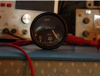
You can see that the duty cycle has reached 100%. I could not get the gauge to read higher than this, even with the pressure pumped up well over 100PSI.
