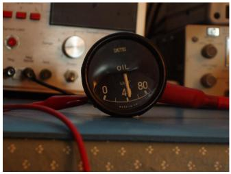
You can see that the increasing duty cycle increases the average amount of current flowing through the gauge.
