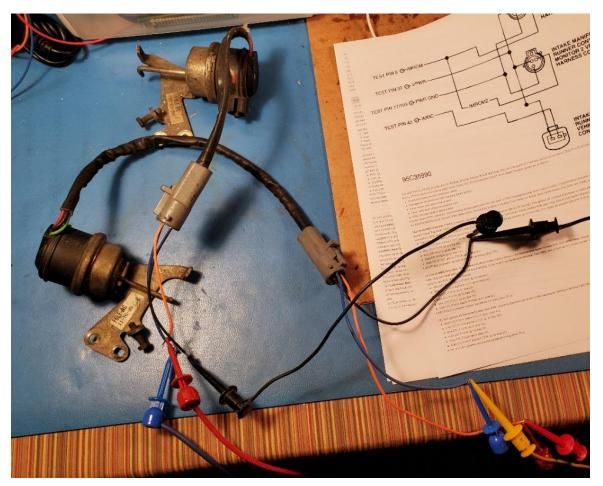
The IMRC system in the 1996 Lincoln Mark 8 is made of single year parts that are getting harder and harder to find. This document describes how the system works and how to use a simple automotive relay to prevent a check engine light if the IMRC system is deleted. Other Ford vehicles such as the Windstar also use this style system, so this information may apply to them as well.
