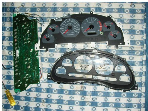
13. Carefully remove the needle from the gauge you are calibrating using a dinner fork.
