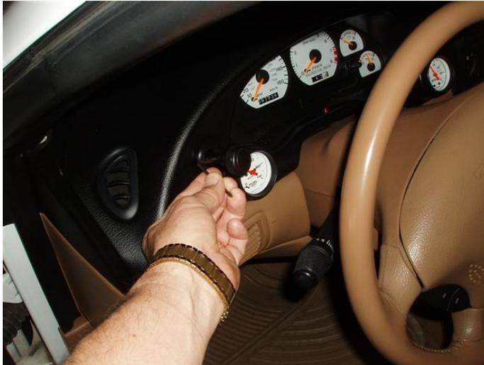
3. Remove the screws that hold the instrument cluster bezel on.
