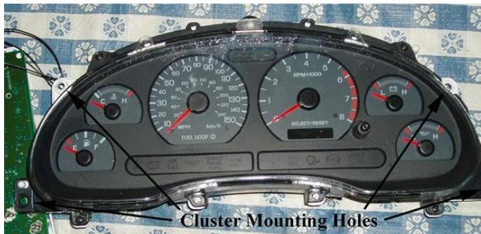
6. Carefully pull the cluster out far enough to disconnect the two cluster wiring connectors one on either side of the back of the cluster. Unhook the boost line from the mechanical boost gauge in 03/04 Cobras.
