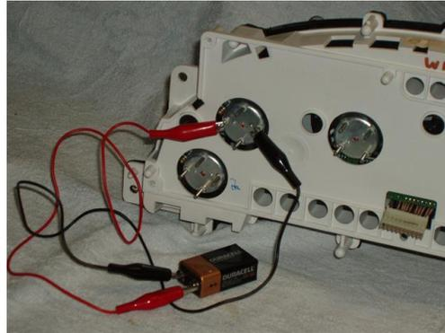
16. If you are calibrating a major gauge, connect the positive lead to one of the bottom gauge pins and add another clip-lead to connect the second bottom pin to the first bottom lead. Connect the negative lead to one of the top gauge pins and add another clip-lead to connect the second top lead to the first top lead. This will center the major gauge meter movement.
