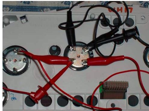
17. With the needle centered on the gauge, carefully push the needle onto the meter movement until it is firmly on the meter post. Don't push it down too far or the needle will bind on the gauge faceplate, causing the gauge to not work properly. This example shows calibration of the voltage gauge.
