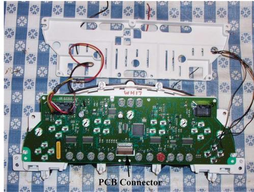
10. Unplug the electrical connector at the bottom center of the cluster. Pull the Printed Circuit Board from the gauge connector pins and remove the PCB
