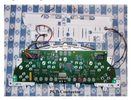
10. Unplug the electrical connector at the bottom center of the cluster.
