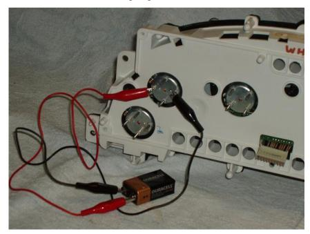
16. With the needle centered on the gauge, carefully push the needle onto the meter movement until it is firmly on the meter post. Don't push it down too far or the needle will bind on the gauge faceplate, causing the gauge to not work properly. This example shows calibration of the voltage gauge.
