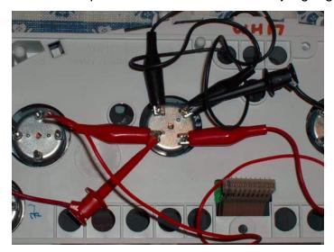
18. With the needle centered on the gauge, carefully push the needle onto the meter movement until it is firmly on the meter post. Don't push it down too far or the needle will bind on the gauge faceplate, causing the gauge to not work properly. This example shows calibration of the speedometer.
