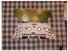
11. Remove the screws that hold the plastic cover on the front of the cluster
