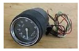
tachometer. The rear case cover simply pops off to provide access.
