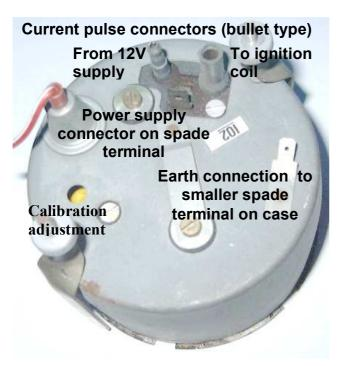
Gen-2 tachometers have the whole pulse coil assembly inside the case with connections brought out to bullet connectors as shown.
