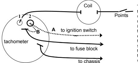
This should have the tachometer displaying rpm with the engine running. If not, check first for smoke (supply polarity wrong) then for 12 volts between the case and the spade terminal. If this is OK then swap connections to terminals 1 and 2. If the tachometer is still not working then it needs repair.
