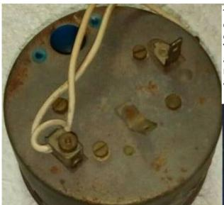
This is the Gen-1 OEM tachometer which has one of the power supply connections electrically connected to the metal case. In many cases the "red-line" will be marked on the dial but not always. Similarly, polarity will be generally be marked on the dial as shown but this also may not always the case.
