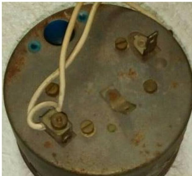
This is the Gen-1 OEM tachometer which has one of the power supply connections electrically connected to the metal case. In many cases the "red-line" will be marked on the dial but not always. Similarly, polarity will be generally be marked on the dial as shown but this also may not always be the case.
