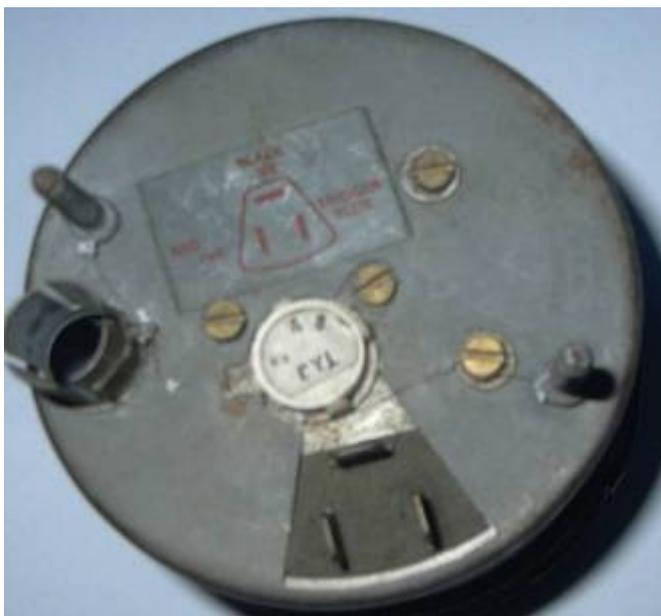
Note the white selector switch above the terminals. This selector switch is only found on Gen-4 instruments, Gen-3 RVC tachometers used a switch accessed through a hole in the rear of the case. The lower picture is a close-up of the label setting out the connections for all these instruments.
