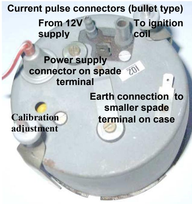
Gen-2 tachometers have the whole pulse coil assembly inside the case with connections brought out to bullet connectors as shown.
