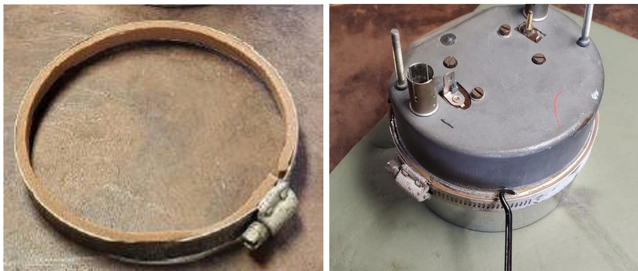
FIGURE C.1: Tool for removing spun-on bezel. A strip of adhesive backed foam rubber is stuck to a worm-drive hose clamp which is clamped around the rim of the bezel. The rubber is to protect the finish on the bezel itself. A blade screwdriver or similar is used to lift the spun over metal to remove the bezel. Right hand photograph shows tool fitted to a Volvo RVI 3410/00 tachometer.
