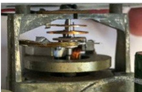
FIGURE F.2: Early meter assembly showing the die cast bridge that is part of the meter body casting. Circled area in right-hand picture shows solder added to the meter armature counterweight to balance the assembly.
