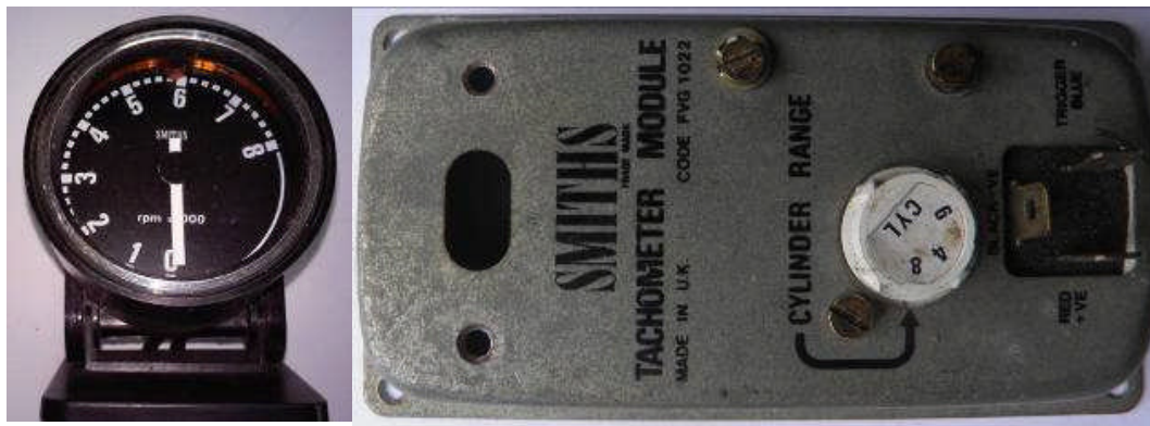
FIGURE 6.6: Gen-4 pod style tachometer comprising FVG 1021 head unit and separate FVG 1022 electronics module for mounting under dashboard.
