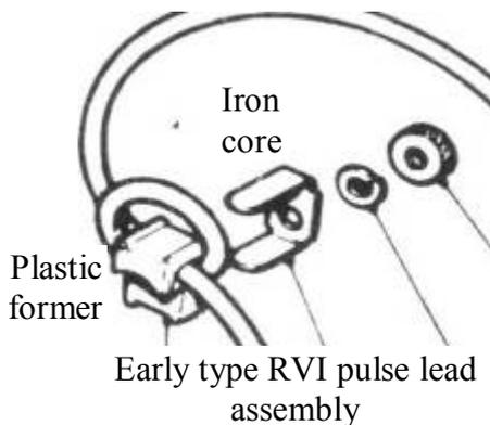
A most important piece of the pulse lead assembly of the early RVI tachometer is the "Iron core". Without it, the tachometer will not work! One could easily be made if required. This "little bit of tin" completes the magnetic circuit that allows the tachometer to sense pulses. ***It is a fairly simple matter to make a new iron core. See Appendix C to this document for details.***
