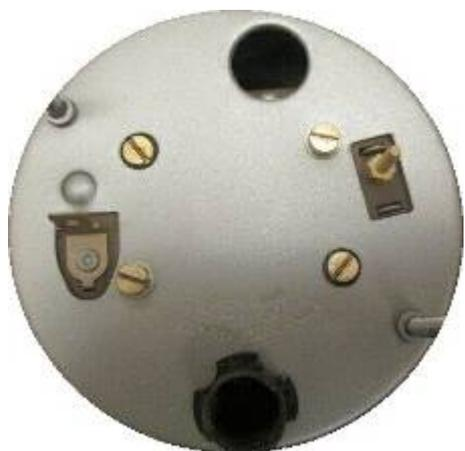
This is the Gen-1 OEM tachometer which has one of the power supply connections electrically connected to the metal case. In many cases the "red-line" will be marked on the dial but not always. Similarly, polarity will be generally be marked on the dial as shown but this also may not always be the case.
