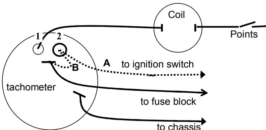
This should have the tachometer displaying rpm with the engine running. If not, check first for smoke (supply polarity wrong) then for 12 volts between the case and the spade terminal. If this is OK then swap connections to terminals 1 and 2. If the tachometer is still not working then it needs repair.
