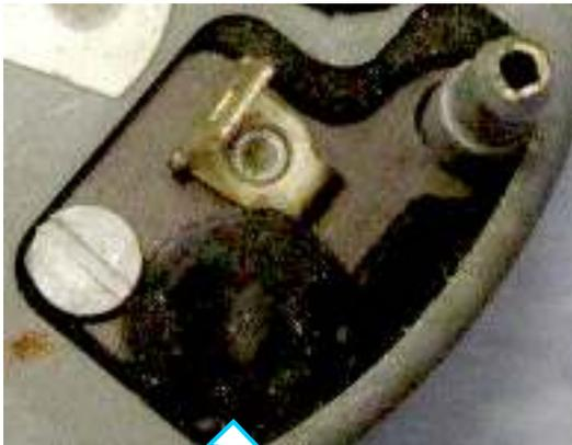
Rubber plug here in lieu of female bullet connector on the RVI tachometer.
