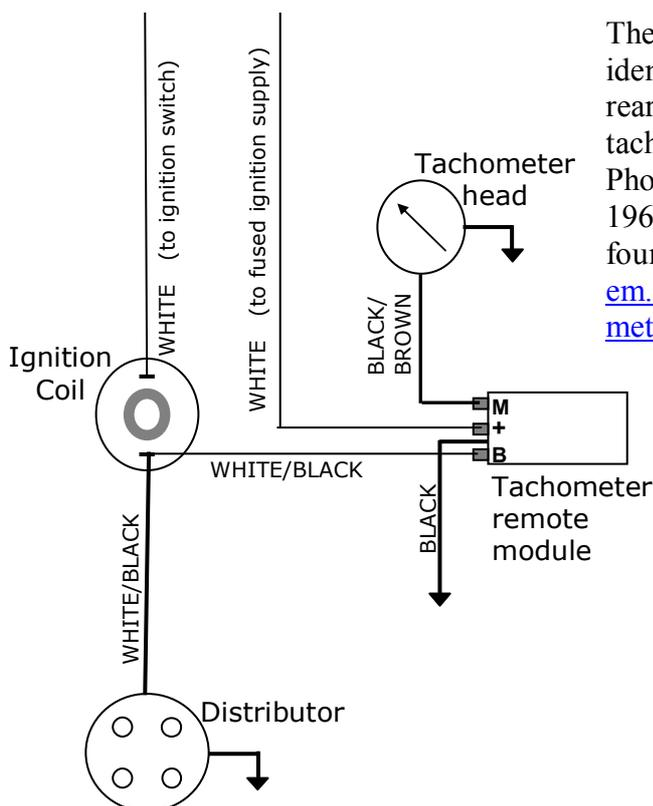
The tachometer head of these instruments can be identified by the presence of two blade connectors on the rear of the case as the only electrical connections to the tachometer.
