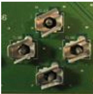
Check the pin-to-PCB gaps
