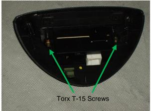
Remove the two Torx T-15 screws and the clock module will come free from the clock pod. You may want to tape your clock connector down so it will not get lost inside the dash while you install the ClockGauge.
