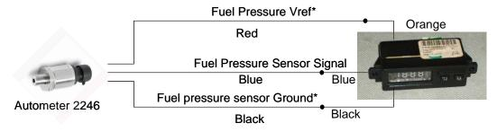
\* Do not connect these wire to the sensor pigtail if you are already running the Autpmeter fuel pressure gauge.
