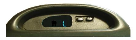
If you choose the Low intensity display mode, the clock gauge will dim the display when the car's lights are turned on.
