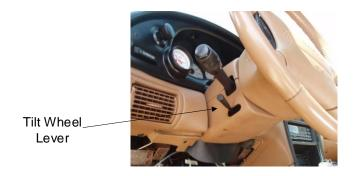
Remove the 4 Philips screws from the bottom of the steering column cover:
