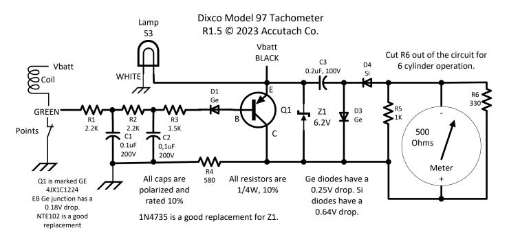
The first model 97 I looked at has basically the same circuit as the Model 797, with different values for three components, R4, R6 and C3.
