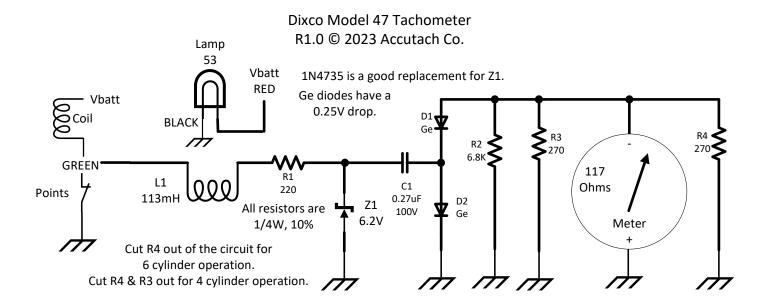
I also reverse engineered a Dixco Model 47 tachometer marked #7 which does use a transistor. The circuit is similar to that of the Model 97s. Here are the schematics for that unit:
