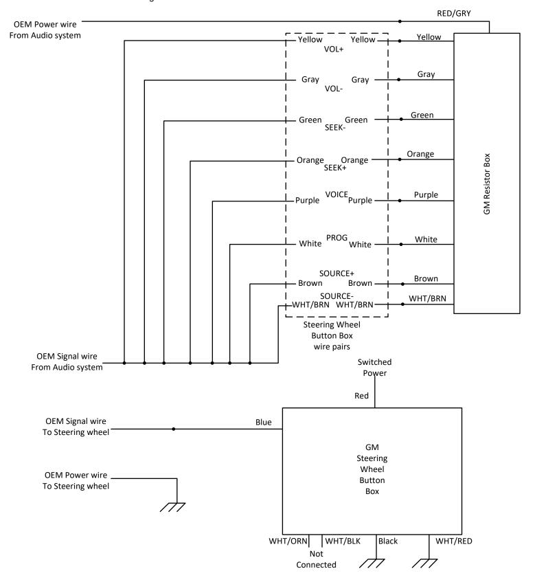
To repurpose any of your buttons, simply don't connect the colored wire pair for each repurposed button to this circuit. Connect those wire pairs to the accessory that you want to control.
