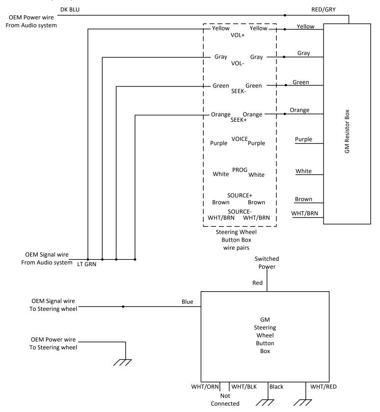
The Purple, White, Brown and WHT/BRN wire pairs can then be wired to control your racing accessories with the VOICE, PROG, SOURCE+ and SOURCE- buttons respectively.
