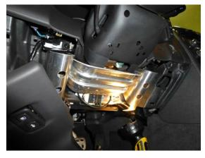
Find connector C231 behind the metal panel. Slide it left to release it in order to get access to the steering wheel control signal wire. It should look like this:
