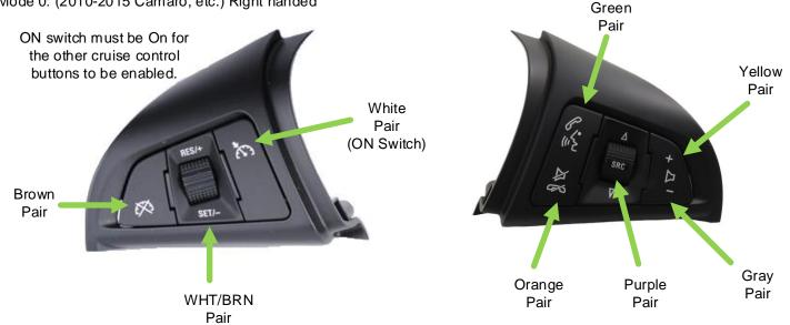
Mode 0 is selected by leaving the WHT/ORN & WHT/BLK wires disconnected. Put shrink tubing over the ends of these wires to ensure they don't accidentally short to anything.
