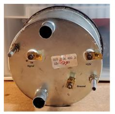
Connect the adapter's Blue wire to your vehicle's tachometer signal. Connect the adapter's White wire to the vehicle's tachometer signal input. Connect the adapter's black wire to a good ground and connect the adapter's red wire to a switched power source. Reconnect your battery and test the installation.
