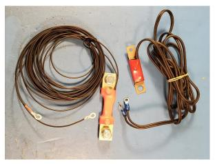
The large metal terminals on the shunt carry the current from the alternator to the battery. The two wires carry the current that drives the ammeter gauge.
