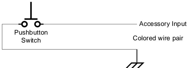
If you are using the pushbutton to control power to an accessory, you will need to connect one of the colored wires to a power source and the other to the accessory input. If the accessory draws more than 1 amp of current, you must use to Steering Wheel Button Box output to control an automotive relay.
