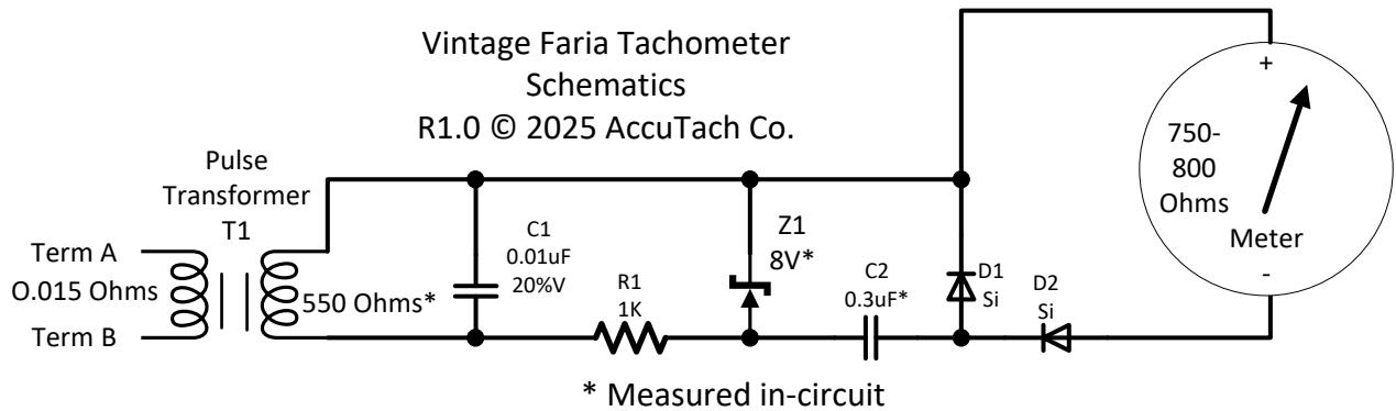
When the top of T1 is negative, C2 is discharged through D1, with no current flowing through the meter. When the top of T1 goes positive, C2 is charged to 8V through the meter and D2, deflecting the meter. Z1 ensures a consistent charge of energy for each pulse by limiting each charge to 8V. Here is a shot of the voltage across Z1 being limited to 8V:
