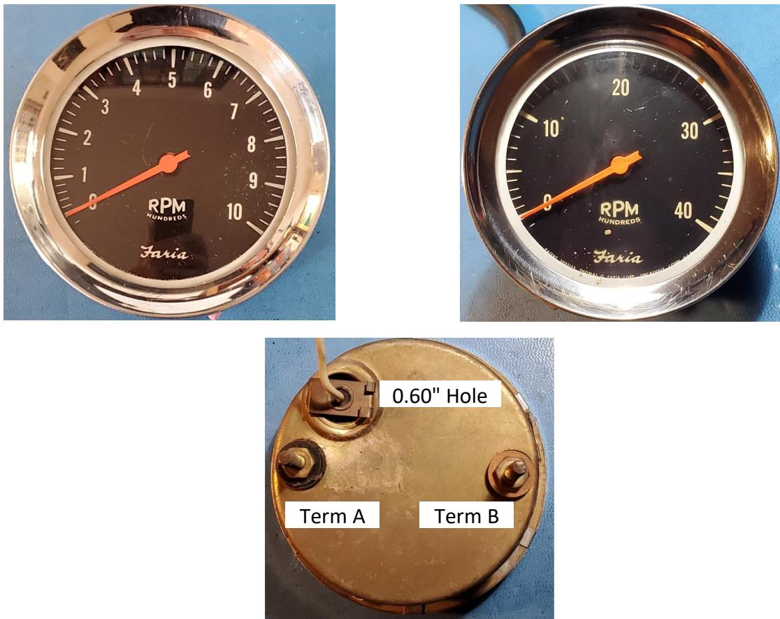
All of the vintage Faria tachometer documentation on the internet indicates that the Faria tachometers are wired between the ignition switch and the coil positive, which implies that they are current driven tachometers. There also is no indication that the tachometers are polarity sensitive since there is no information differentiating between the two terminals. I have arbitrarily marked the terminals A and B.
