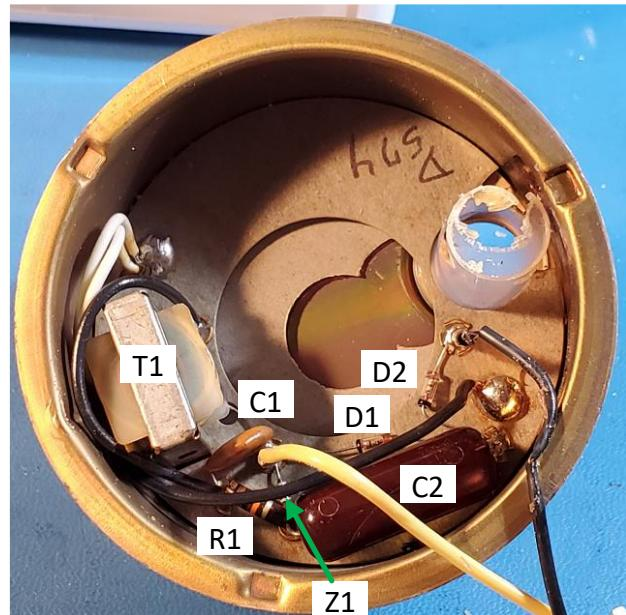
Note: The circuit board is riveted to the back of the case. Here are the schematics of the tachometer circuit:
