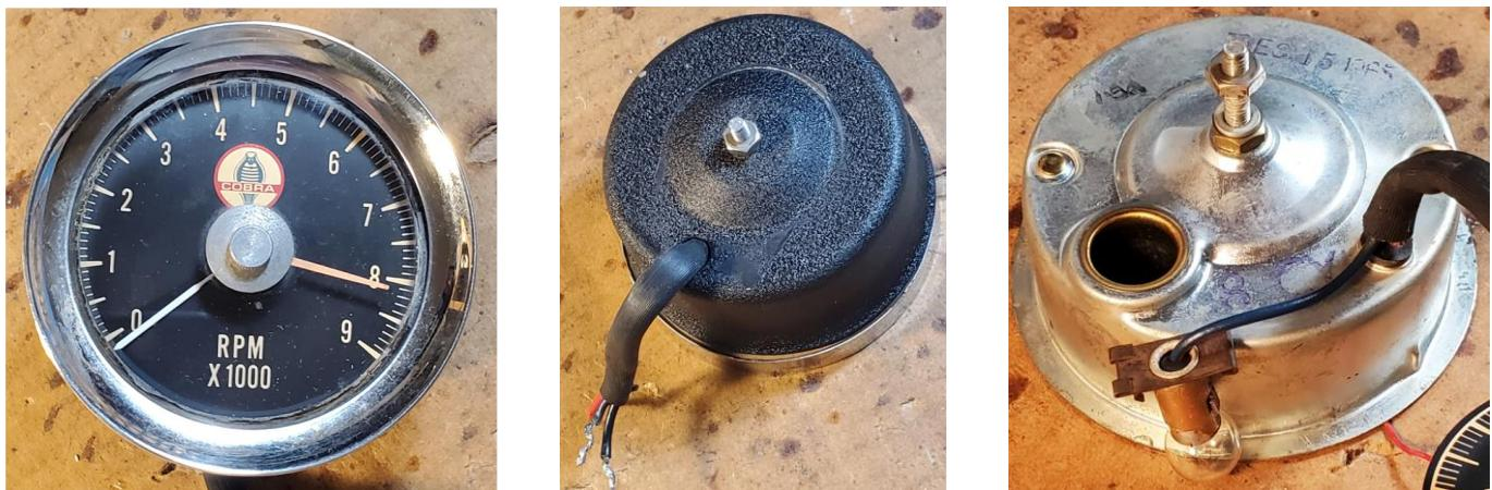
It is a little different from the other Faria tachometers in both the circuit and the tachometer connections. The previous tachometers had two stud terminals on the back of the case whereas the GT350 unit has two wires going through a strain reliever on the back of the case.
