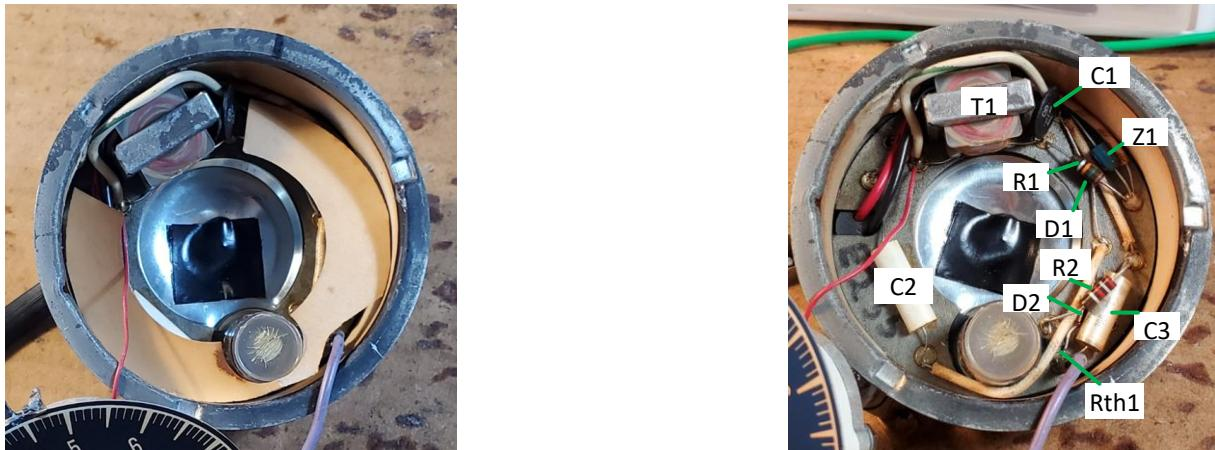
The circuit is very similar to the circuit in the 4K tachometer with the addition of some thermal compensation components. C3, R2 and Rth1 change resistance with temperature to compensate for the change in resistance of the copper deflection coil with temperature.
