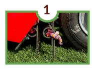
The tines on the front of the machine have adjustable depth, and serve to de-compact the top inch of the playing surface.
