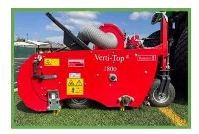
The Redexim Vertitop 1800 is a comprehensive cleaning system designed specifically for synthetic turf fields. Our experts recommend cleaning your turf one to two times per year to maintain its condition and safety.
