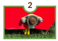
The powered brush collects small debris and trash while the sieve behind it allows any rubber infill to return to the playing surface while a powerful vacuum system collects particles such as dust and hair.
