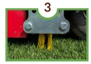
On the back end, an adjustable broom is lowered to groom the fibers and leave each pass with an attractive and clean stand of turf.
