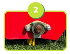
The powered brush collects small debris and trash while the sieve behind it allows any rubber infill to return to the playing surface while a powerful vacuum system collects particles such as dust and hair.
