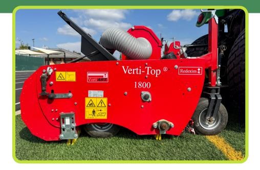
The Redexim Vertitop 1800 is a complete cleaning system for synthetic turf fields.
