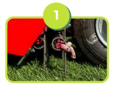
The tines on the front of the machine have adjustable depth, and serve to de-compact the top inch of the playing surface.
