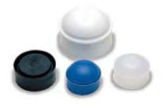
Cartridge plungers ensure that the pressure is evenly spread across the fluid surface to provide consistent dispensing. Wiping edges prevent dripping and eliminate material waste by wiping the cartridge walls clean, as fluid is dispensed. The plunger is inserted into the cartridge once filled (or supplied pre-inserted when bottom filling) and it moves down the inner walls under pressure to ensure all liquid material is dispensed without waste.
