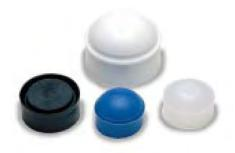
Cartridge plungers ensure that the pressure is evenly spread across the fluid surface to provide consistent dispensing. Wiping edges prevent dripping and eliminate material waste by wiping the cartridge walls clean, as fluid is dispensed. The plunger is inserted into the cartridge once filled (or pre-inserted when bottom filling) and it moves down the inner walls under pressure to ensure all liquid material is dispensed without waste.
