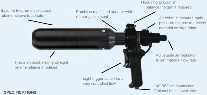
Maximum Thrust: 2.5kNBarrel Length: 383.2mmPressure: To 100 PSI
