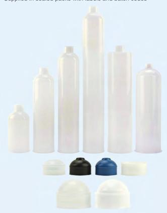
Disposable dispensing cartridges are also available in 2.5, 6, 8, 10, 12, 20 and 32 oz. (approximate metric value 75cc, 177cc, 237cc, 310cc, 355cc, 591cc, 960cc). Available in the highdensity natural polyethylene (HDPE) which is more rigid material and also low density polyethylene (LDPE) which is a softer grade material. Other colours are available.
