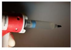
Remove the tip cap from the tip end of the 10cc barrel. This will expose a male luer lock thread on the barrel ready to accept any of our dispensing tips.
