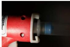
Align the barrel flange to the gun flange. Push over rod end and over O-ring seal. Push all the way and then twist the barrel anti-clockwise.
