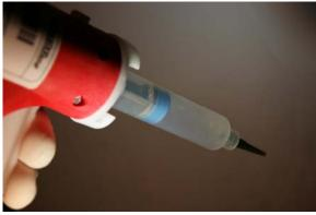
Hold the gun and position the tip above the area to be dispensed to. Squeeze the trigger to make a deposit. Release the trigger to stop. For the best results, touch the tip to the surface of the part, make deposit then release trigger before moving the gun away. This will release all the fluid to the part and not carry over or spill from the tip when finished. Ensure the piston does not have an air gap between the fluid or it might drip.
