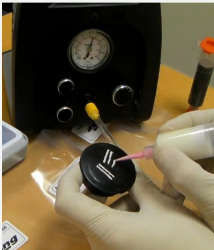
The TS250 is a digital timed air powered dispenser. It's small footprint makes this the ideal bench top solution for all your gluing, solder paste application and most other fluids. Its digital timer and shot counter replaces squeeze tubes, bottles, brushes and syringes. The TS250 comes with two modes; manual and pre-set timer.
