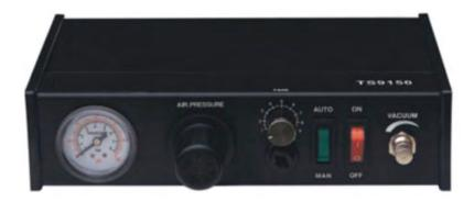
The TS9150 is a simple dispensing system for applying watery liquids to high viscosity pastes. It has a traditional design with hard metal case and runs a super quiet operation. Used for applying small dots and controlled beads of materials direct from industrial syringe barrels or can be used as a valve controller with the foot switch connector modified by the customer as required.
