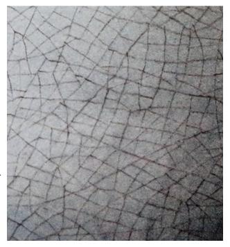
When gelcoat cracking is a symptom of another problem, repairing the crack and not repairing the underlying cause could lead to repeated cracking. In the case of a thick gelcoat, thinning the gelcoat is not practical.
