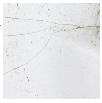
wet cloth so the cracks or fractured fiberglass will appear as white lines in the laminate.
