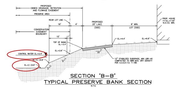
The above cross section shows the bottom of the open-water channel elevation at -4.6 feet and the Control Water Elevation at +2.4 feet. Based to this cross section, the bottom of the open water channel was designed to be 7 feet below the Control Water Elevation. The design documents also contained the following drawing. (The A & B cross-sections are shown on the following page.)
