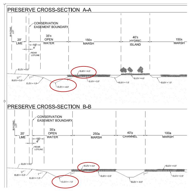
The Preserve Cross-Section A-A above shows the open water channel elevation at -6.0 feet and a line that appears to be the Control Water Elevation at +4.0 feet; thus, indicating a designed water depth of 10 feet. Additionally, the Preserve Cross-Section B-B above shows the open-water channel elevation at -1.6 feet and a line that appears to be the Control Water Elevation at +4.0 feet; thus, indicating a designed water depth of 5.6 feet.
