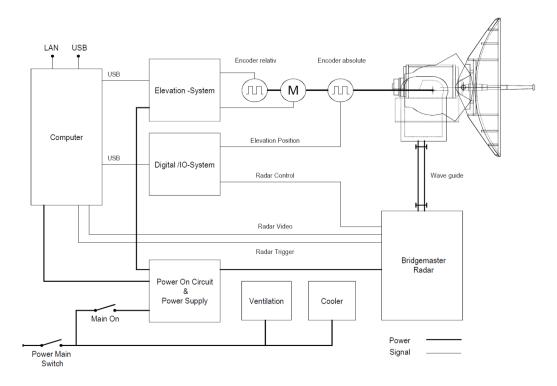
The computer for control of the system is BookSize PC of DSM Computer. The video signal of the radar is digitized at 12 MHz frequency and is processed by specially developed BirdScanMS1 software.
