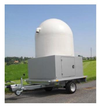
The antenna allows movement along horizontal and vertical axes with directing to the sector that requires monitoring. The angle can be changed in a certain range (0 to 90 degrees). It is positioned across the main migration stream in St. Nikola Wind Farm and covers a maximum area along the power plant.
