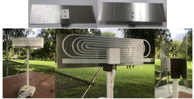
The hole in the 5 ½" x 5 ½" x 1 ½" wooden base and the shield for table top mount is 7/8" or 22mm.
