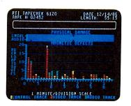
Color coded bar graphs present magnetic and physical evaluation results in easy to read format. Six different time scales can be selected.
