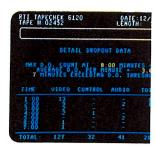
Tabulates dropout counts fo every minute of the tape. Provides actual counts for critic detailed analysis.
