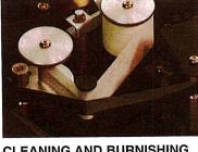
**CLEANING AND BURNISHING** The TapeChek cleaning and burnishing system extends the life of your tapes. Improves tape performance. Minimizes VCR maintenance. Uses a special automatic advancing cleaning tissue. Has a "Replace Tissue" warning system.
