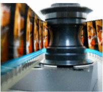
The film rolls have been specially designed so to touch film only at perforation edges and are provided with tin-like ball bearings to avoid film stress and damage.
