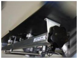
For a correct adaptation of the equipment to the fragility of the loaded film, a tension control is provided.
