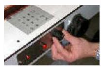
A checking-speed selector grants three adjustable constant speeds for each direction. The standard setting (12fps-24fps-150fps) can be easily changed by the operator directly from the setting menu on the keyboard.
