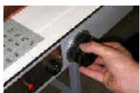
An easy and ergonomic control knob enables the operator to run the film in either direction with variable speed from 0 up to 200fps (max peak speed) maintaining always the same tension during all the operations.
