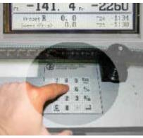
The digital counter measures in real time the film length in feet, frames, meters, fps and elapsed time at 24 or 25 fps and the operator can locate a certain frame simply digiting its foot and frame references on the keyboard.
