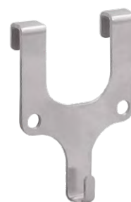
Painting hook INOX type L, with 2 holes for fixing on the lower wire, load capacity up to 70 kg
