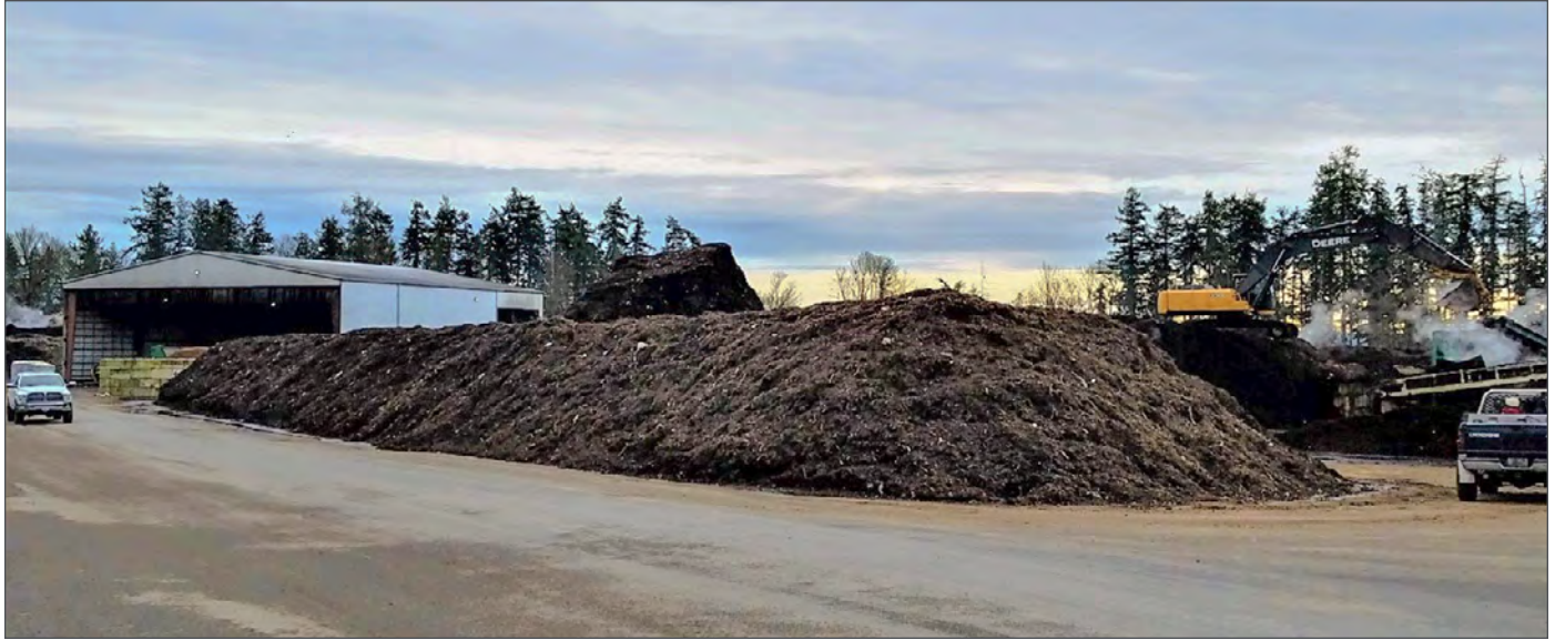
Figure 2.5. Integrating biochar production with commercial compost facilities, like the one pictured, offers promise. Compost facilities have a ready source of woody materials (compost overs) and co-composting with biochar can produce a high-value soil amendment. (Photo: Doug Collins)
