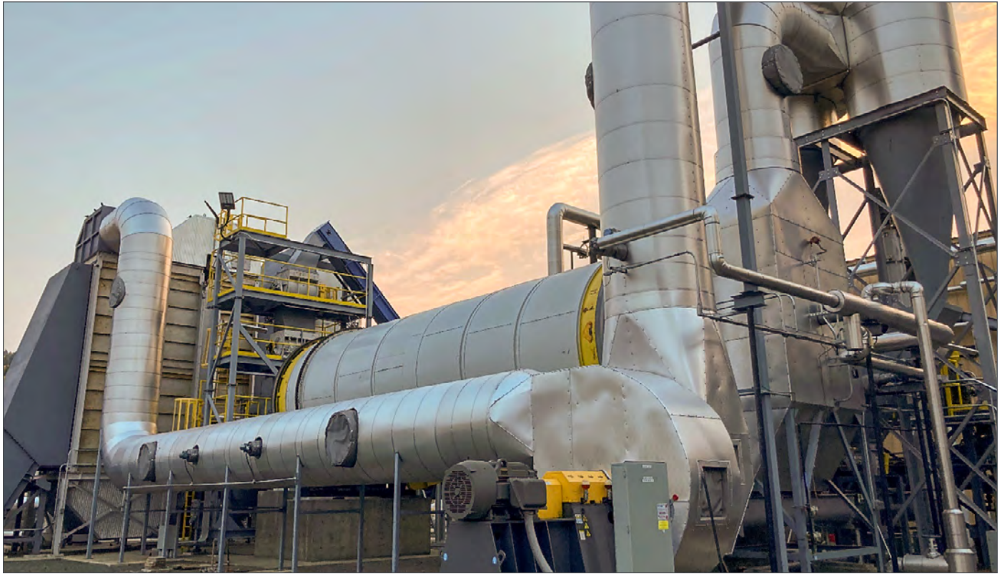
Figure 6.2. Torrefaction system at Restoration Fuels in John Day, Oregon. (Photo: Matt Krumenauer)
