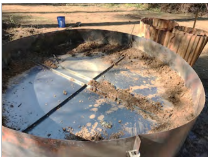
Figure 4.4. Using a lid to snuff quench a flame-cap kiln. (Photo: WilsonBiochar.com)
