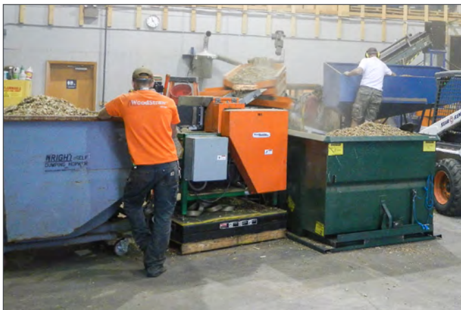
Figure 10.5. Wildfire protection thinnings were used to produce 4mm feedstock for biochar production. In this example, biomass was transported intact for comminution and screening at a centralized facility. (Photo: Forest Concepts)
