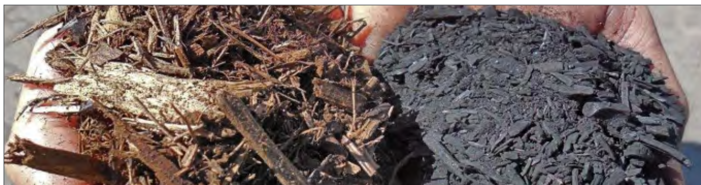
Figure 1.1. Biochar (right) is the carbon-rich solid produced by heating biomass (left) under low-oxygen conditions. (Photo: Biomacon)
