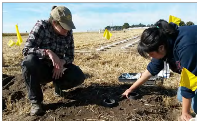
Figure 8.6. Stephanie Chiu and Sarah Light remove soil cores to test the response of soil water to biochar additions at a field trial site in Pendleton, Oregon. (Photo: Claire Phillips)
