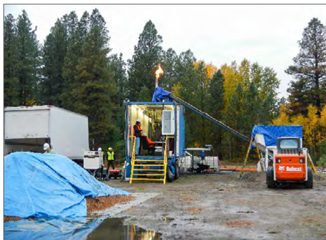
Figure 5.1. Relocatable moderate-scale pyrolysis biochar system with a capacity of approximately one ton per hour of wood chips. (Photo: Jim Dooley)
