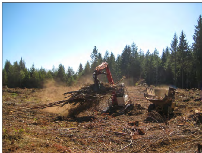
Figure 10.2. Gathering forest residues using a loader and a modified dump truck on a recent timber harvesting site near Humboldt, California. (Photo: Han-Sup Han)
