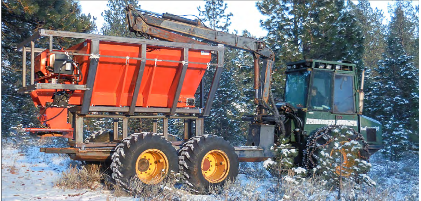
Figure 2.2. The USDA Forest Service National Technology Development Center developed a biochar spreader that can be used to apply biochar to log landings or skid trails, seen here working on the Lubrecht Experimental Forest in Montana. This equipment can work on slopes up to 35%. (Photo: USDA Forest Service)
