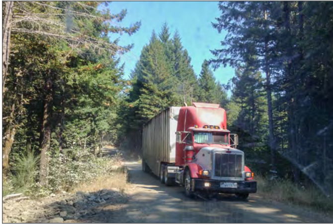
Figure 10.4. A chip van transporting biomass feedstock from a comminution site in the woods near Humboldt, California to a biochar production facility. (Photo: Han-Sup Han)
