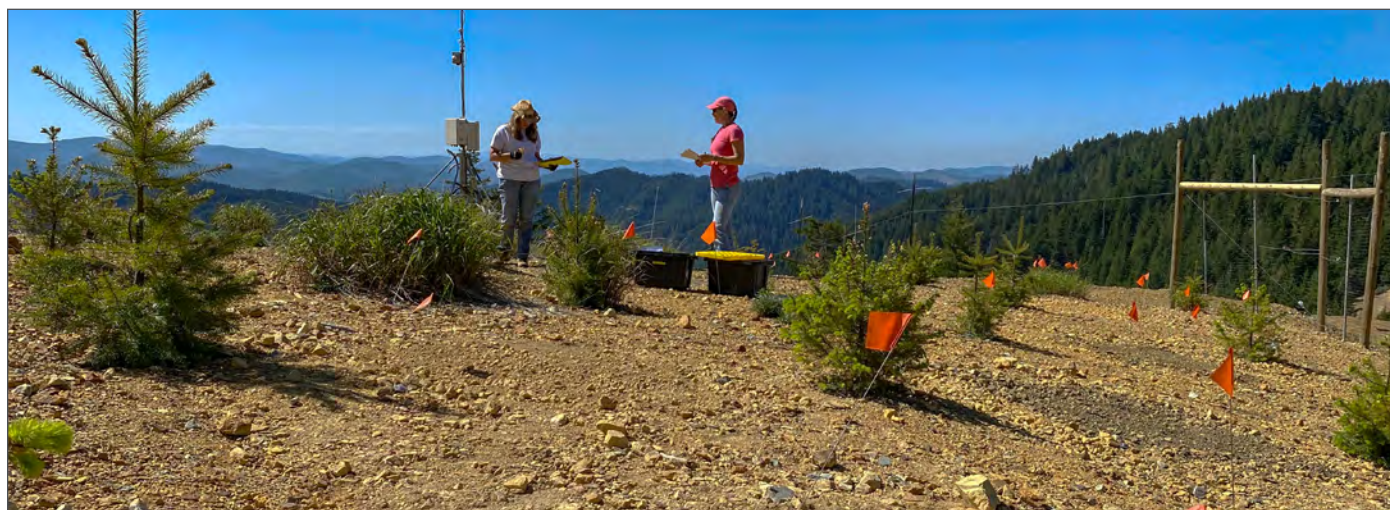
Figure 5.5. Researchers test whether the addition of biochar helps establish vegetation at the Formosa mine site in Riddle, Oregon. (Photo: Kristin Trippe)
