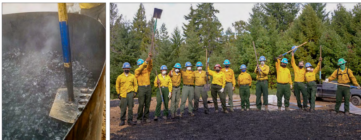
Figure 3.8. A California Conservation Corps crew makes biochar in the Usal Redwood Forest. A McCleod tool is used to level the biochar in the kiln (left) so workers can measure the height of the pile. The CCC crew reacts to the information about how much carbon they sequestered that day (right). (Photos: Wilson Biochar Associates)
