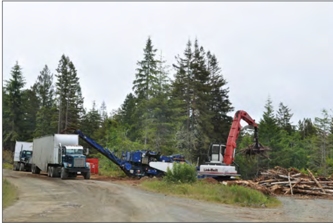
Figure 10.3. A grinder (center) comminuting logging slash and directly loading ground materials onto a truck near Humboldt, California. (Photo: Han-Sup Han)
