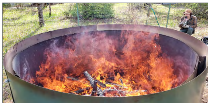
Figure 4.2. Backyard biochar production using the Ring of Fire flame-cap kiln in April 2020 in Cave Junction, Oregon. Counterflow combustion keeps the flame length low and holds heat in the kiln for greater efficiency. Most of the smoke generated is burned in the kiln. (Photo: WilsonBiochar.com)
