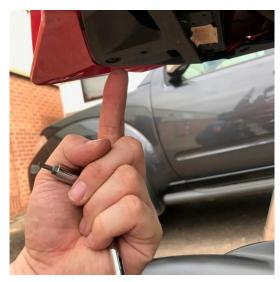
10. REMOVE SCREW FROM UNDER NOSE. 3 SCREWS
