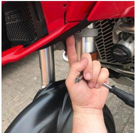
9. REMOVE SCREW FROM UNDER NOSE. 3 SCREWS
