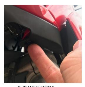
8. REMOVE SCREW FROM UNDER NOSE. 3 SCREWS
