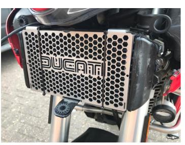
12. GUARD WILL HANG FROM TOP. FOAM WILL PROTECT GUARD FROM RUBBING ON RADIATOR.
