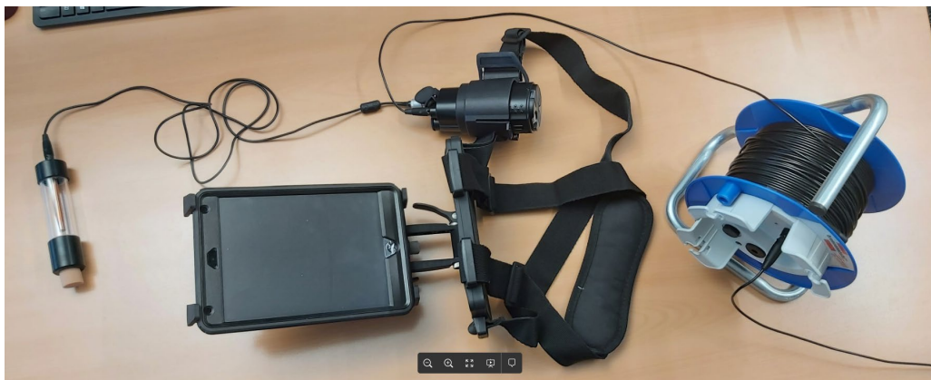
Figure 7 : PM8500 Rod electrode cabling set up
