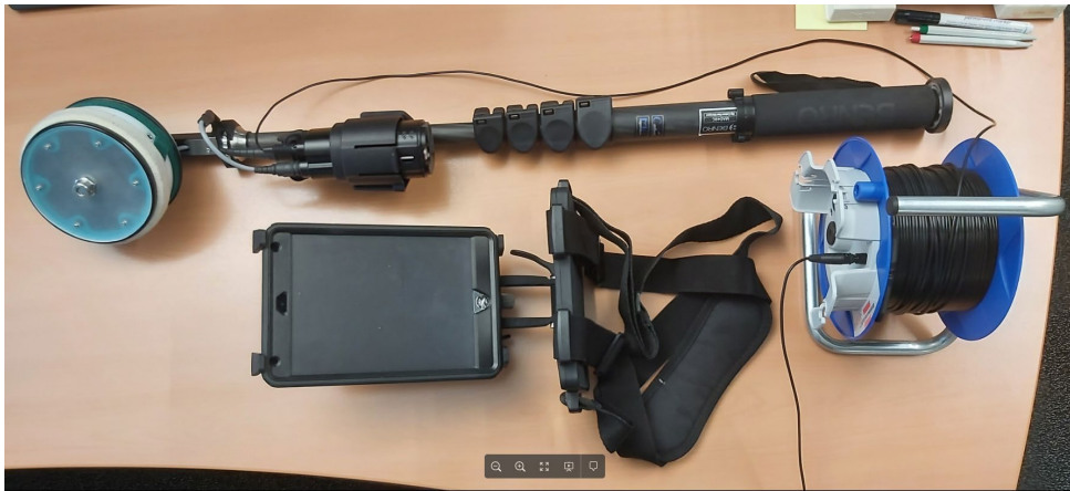
Figure 8 : PM8500 One wheel electrode cabling set up
