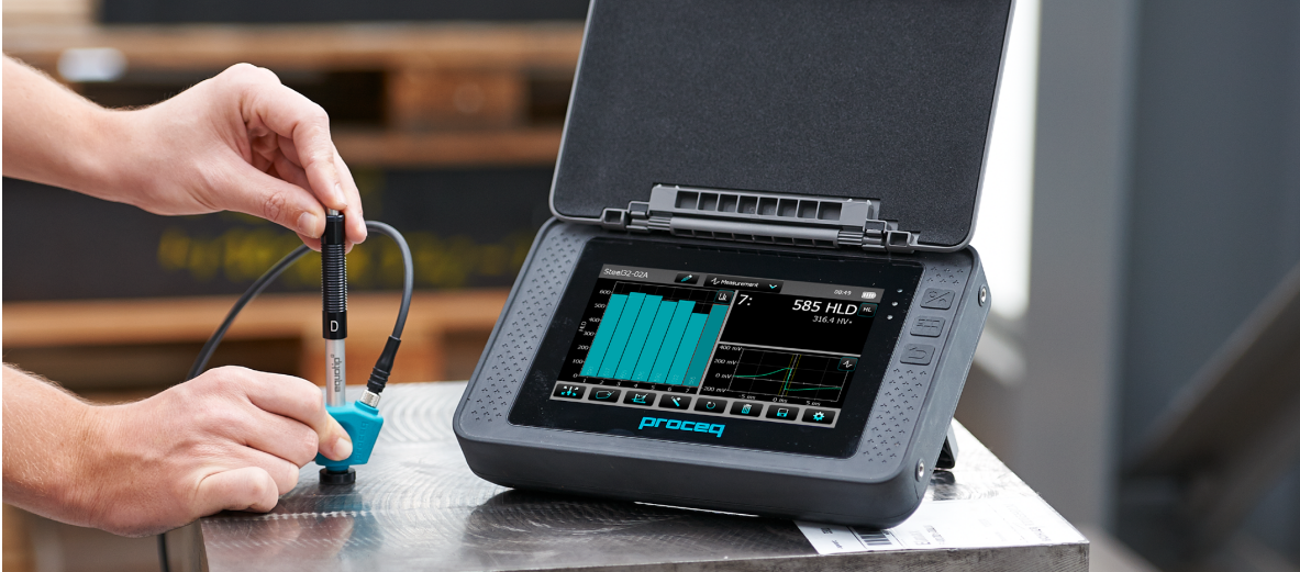
Figure 5: Equotip 550 Leeb hardness testing instrument
