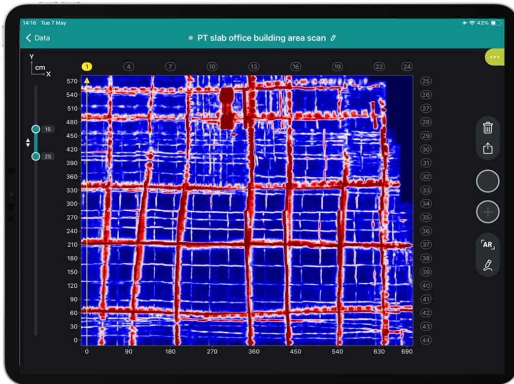
Figure 45: GP app software area scan PT concrete slab application
