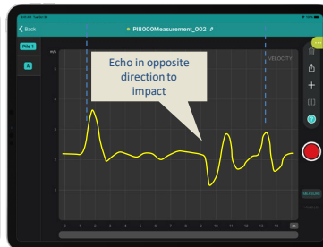
Bulging – increase in diameter
